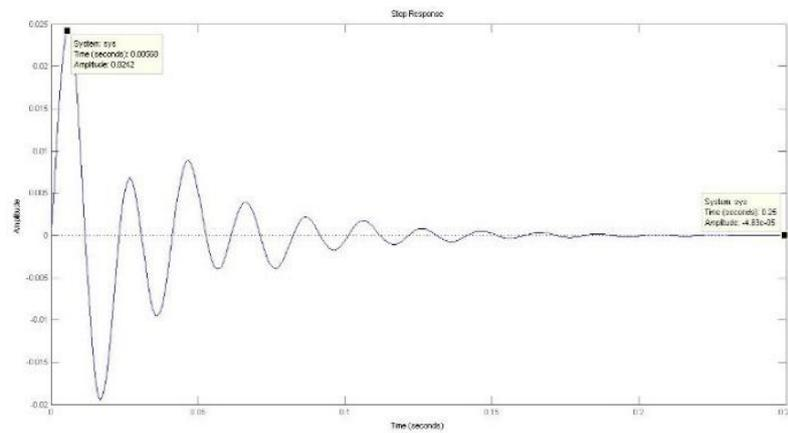
Fig. 6(b) shows the transient response for the 200nF capacitor. For this value of capacitor the overshoot is 77.4% and settling time is 0.25 sec.
