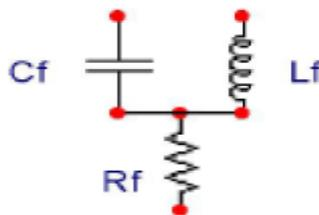
Active Ferro resonance Suppression Circuit contains the parallel connection of Inductor and Capacitor are in series with the Resistor.
