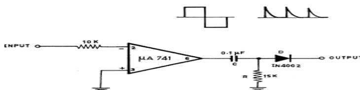
FIGURE 4.4 ZERO CROSS DETECTOR
