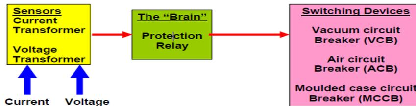
Figure 2.9: Building block of protection system
