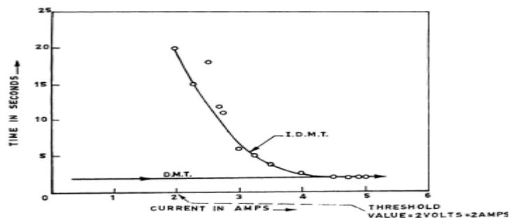
FIGURE 4-12 TIME-CURRENT CURVE OF IDMT AND DMT OVER-CURRENT RELAY
