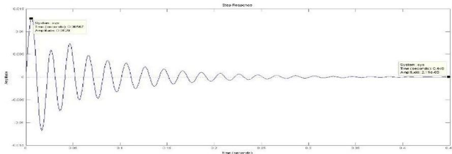
For 100nF value of capacitor, Overshoot is 88% and settling time is 0.449 sec and this transient overshoot are enough to trip the power system relay because the relay are very sensitive to transient.
