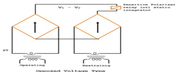
This type works with voltage input signals derived from PTs. The operation depends on the difference of the average **rectified voltage** ( $V_1 - V_2$ ). Here the rectifiers are not protected against higher currents. The relay operates when  $V_1 > V_2$ .
