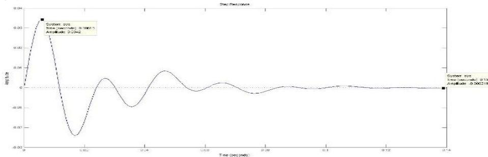
Fig. 6(c) shows the transient response for the 300nF capacitor. For this value of capacitor the Overshoot is 68.1% and settling time is 0.139 sec.
