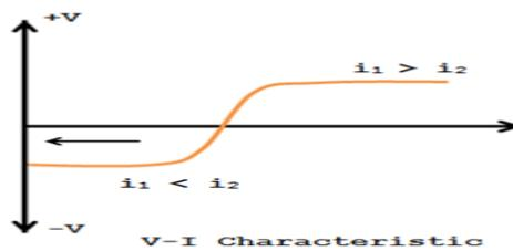
It can also be used as impedance relay. Two rectifier bridges can be arranged in such a manner as shown in the figure below, to function as amplitude comparator circulating type. The polarized relay operates when  $S_1 > S_2$  where  $S_1 = K_1 i_1$  and  $S_2 = K_2 i_2$ . This arrangement gives a sensitive relay whose voltage may be represented in the VI characteristic of the figure.
