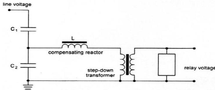
Fig.1. General Structure of CVT
