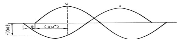
FIGURE 4.3b  $I \cos \theta$  FOR FAULTS IN REVERSE DIRECTION
